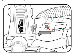
• To release the lock-on, simply push the trigger once, and both buttons will unlock.
