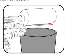
• Once emptied, reseal the bag by sliding the plastic clip back on the bag as it was removed in the first step.
